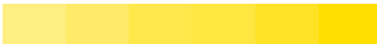
Fig. 7 – The colour range of the solution after the addition of murexide prior to titration
