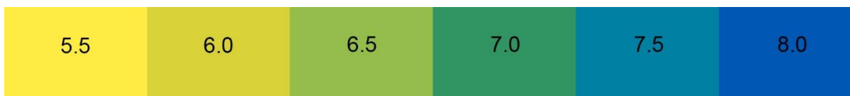
Fig. 1 – The colour range of the solution with bromothymol blue at individual pH
