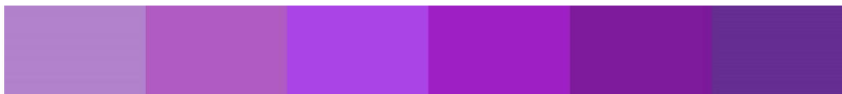
Fig. 4 – The colour range of the solution after the addition of urotropin prior to the titration
