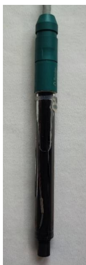
Fig. 2: Photograph and schematic representation of standalone (A) and combined (B) fluoride ion-selective electrodes. The electrode arrangements in the photographs correspond to the schematics.
